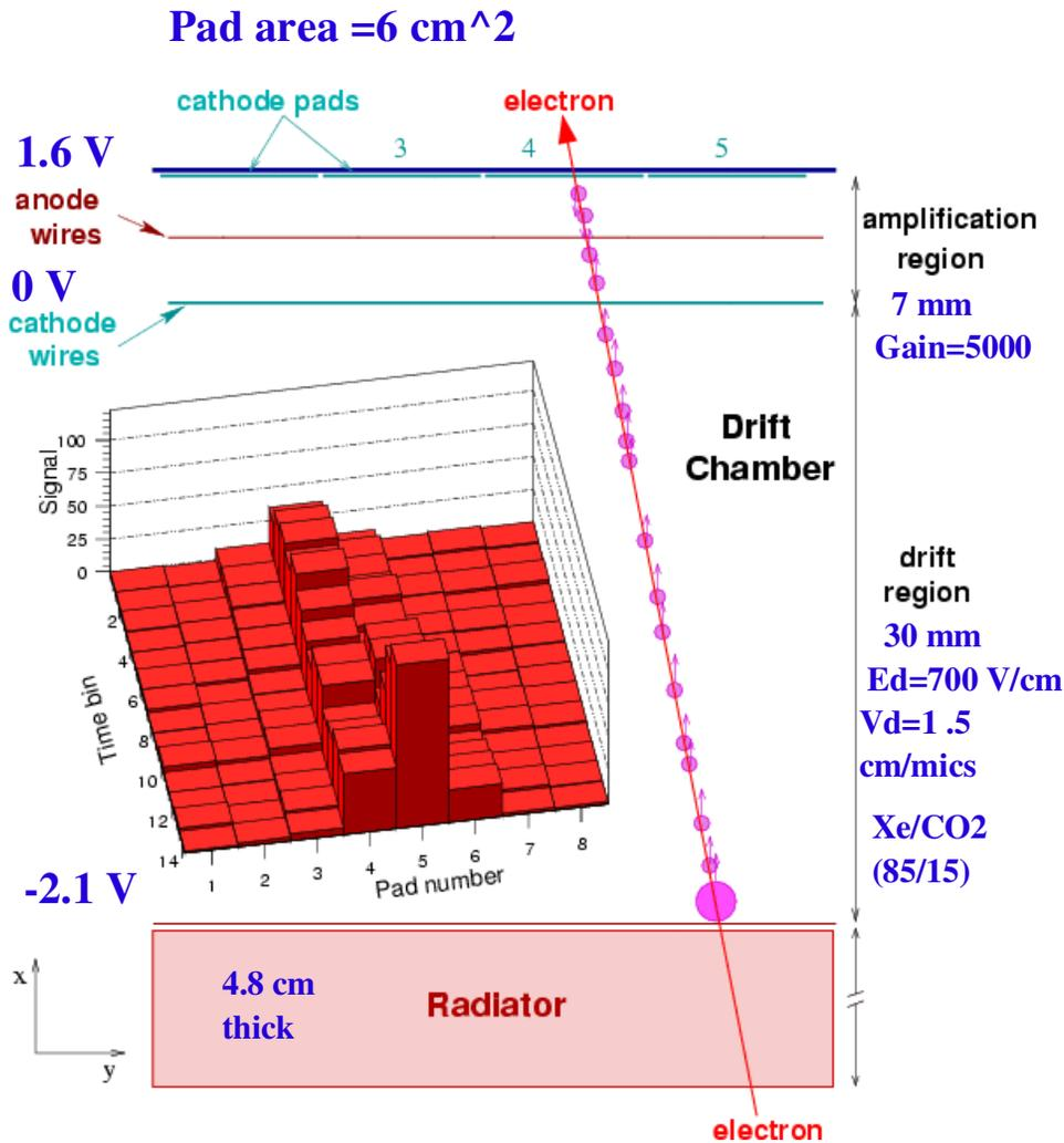
Radiator: fiber / foam sandwich PP,  $17 \mu\text{m}$
