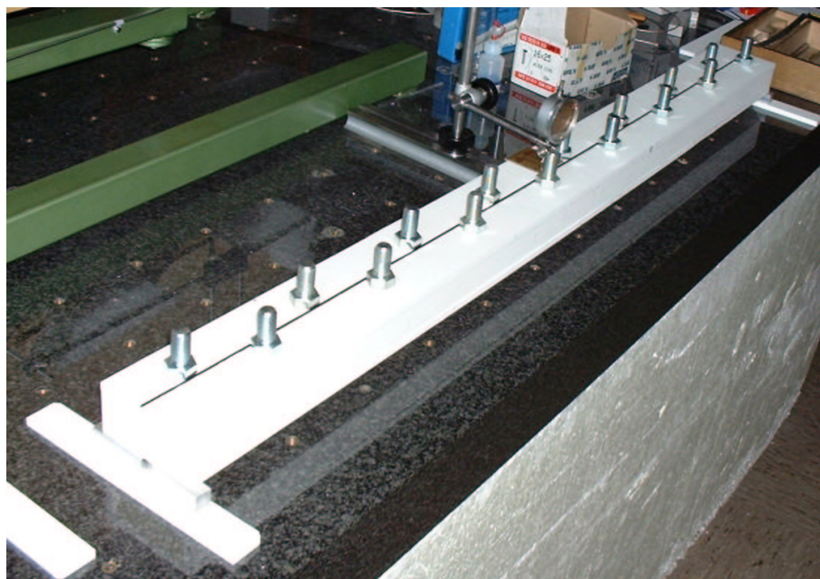
Figure 3.3: The bending test of the reinforced radiator model. One can see the radiator model (white) and the carbon fibre rod (black) glued to it. The overpressure is simulated by weights (in this case screws) distributed over the whole length of the model. The deflection is measured by the dial gauge positioned at the center of the model.
