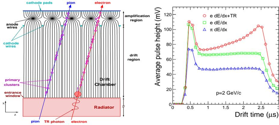
Fig. 1. Detector module is shown on the left with a pion and an electron trajectory. A pulse height spectrum is shown on the right
