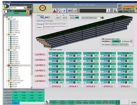
Figure 8: Screenshot of the DCS system for TRD. This example shows the status of the front-end electronics of all 30 chambers within one TRD supermodule.
