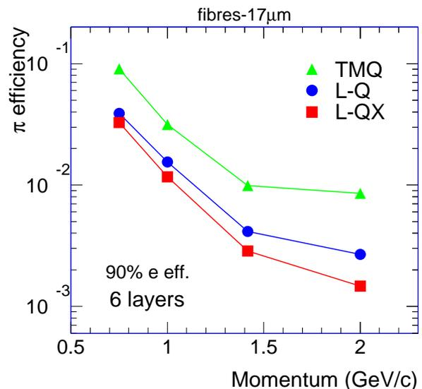
Figure 2: Pion efficiency as function of momentum for a radiator with 17  $\mu\text{m}$  fibres.
