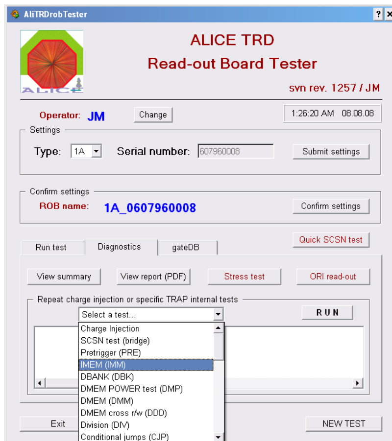
Figure 7.19: Diagnostics panel. From this panel the detailed results of the automatic test are visualized. In addition, it allows to repeat specific tests and perform pre-trigger stress test and ORI readout “manually”.
