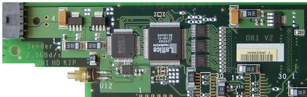
Figure 7.9: The ORI board is mounted as mezzanine board on ROB types 3A and 3B for collecting data from the HCMs and ship them to the GTU over optical fiber at 2.5 Gb/s. It has dimensions 13 \times 4.2 \text{ cm}^2 .
