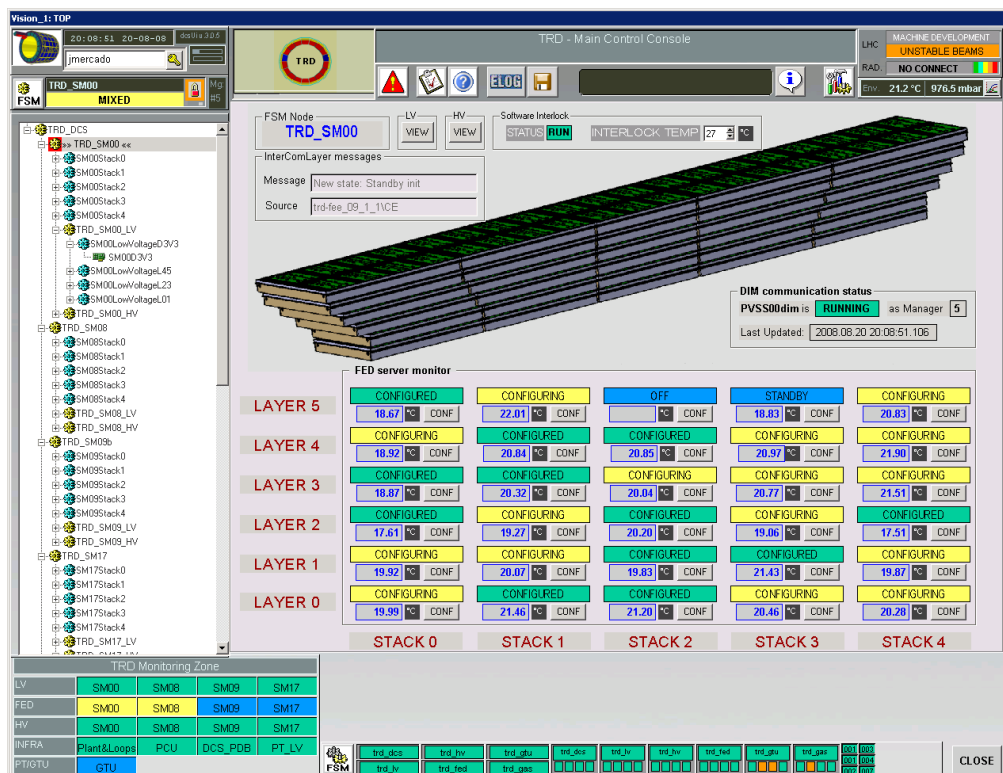
Figure 10.34: GUI displaying the status of all FedServers of one supermodule.
