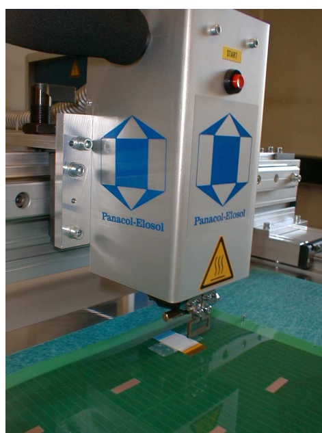
Figure 3.15: Zoom onto the soldering gun. The upside-down- \Omega -shaped head is visible in position right on top of the yellow part of the flat cable.
