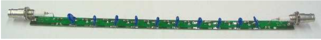
Figure 5.3: Photo of a high voltage filter box. It offers a two stage low-pass filter for up to 8 anode segments and a single stage low-pass filter for the voltage divider in the drift field cage.
