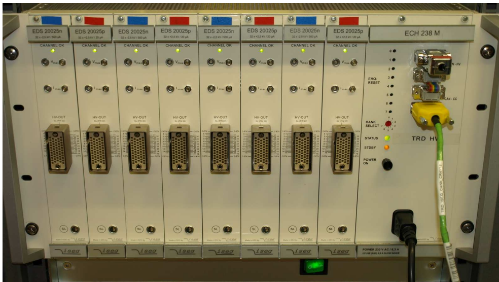
Figure 5.2: Photo of a high voltage crate with eight 32 channel modules.
