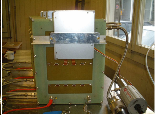
Figure 3.2: The back side view of the prototype TRD. PASA is mounted on the external side of the prototype TRD.
