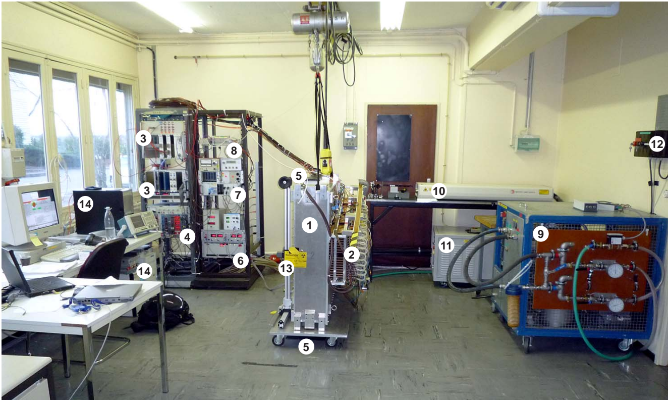
Figure 3.2: Layout of the test setup installation in “LaTotal”: Test box (1) containing the field cage and read-out chamber; support frame with front end electronics (2); high voltage power supplies (3) for field cage, chamber and photomultiplier; NIM electronics (4) used as trigger and calibration pulser; scintillators for cosmic triggering (5); low voltage power supply for electronics (6); gating pulser (7); systems for slow control (8) i. e. temperature, pressure, cathode current, oxygen content, cooling water flow; cooling unit and instrumentation (9), laser head (10) with power supply unit (11) and interlock (12); radioactive source with adjustable support (13); computers (14) for data acquisition, slow control and front end electronics. The gas supply station is not visible.
