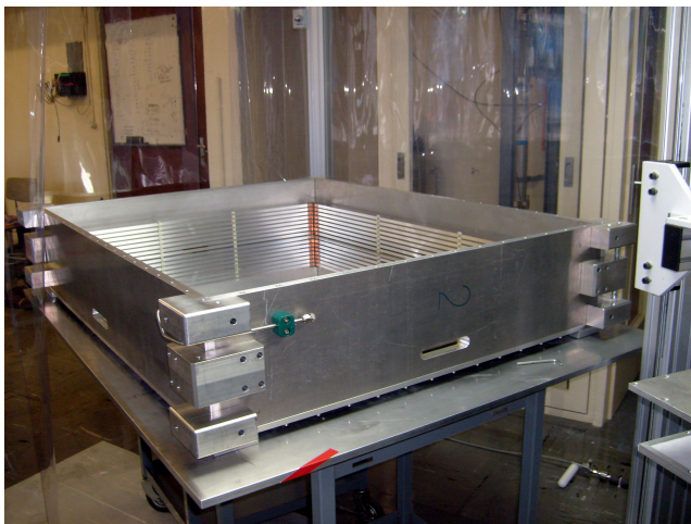
(a) Top plate removed: drift electrode and field strips are visible. On the outside one gas connection and one laser window are seen.
