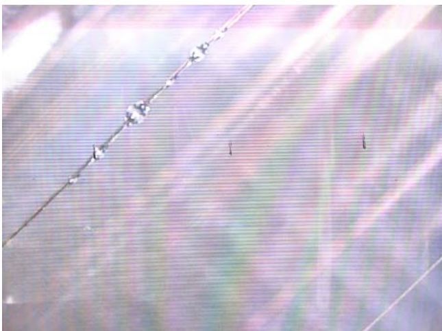
(a) Glue drops on the second edge wire.
